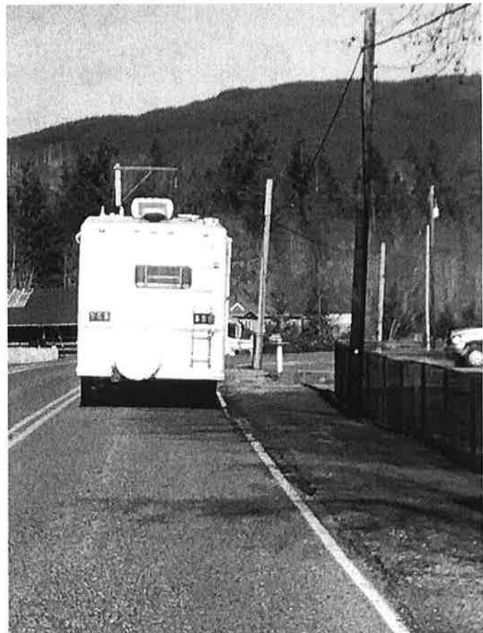
Truck and trailer combination will take approximately 1,774 feet and 74 seconds to accelerate to the 50 mph speed limit.
